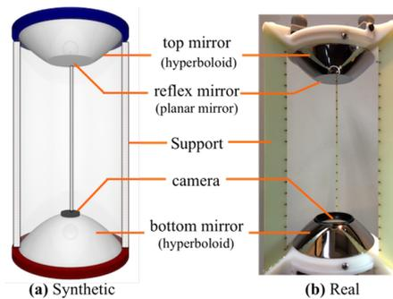
Fig. 1: Single-camera SOS prototypes designed in [1].
