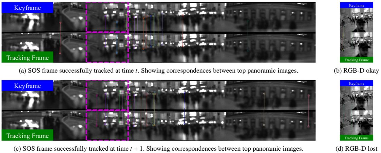
Fig. 7: Example from the stairs sequence at GCT: the single-camera SOS succeeded while the RGB-D sensor failed due to the busy highly dynamic scene diminishing the number of trackable keypoint features when occluded by a sudden passerby in the view. The dotted boxes in the panoramas corresponds to the view in common with the RGB-D.
