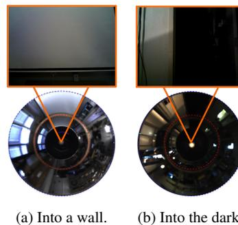
Fig. 5: Illustrating the higher vulnerability that the RGB-D camera (top) has due to the lack of features to track in the scene. The associated omnidirectional images (bottom) have a higher probability to detect features under these special circumstances. Data with these issues are provided in the sequences from the special group of the dataset.
